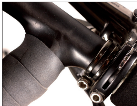
Above, correct lever position on carbon H-Bar™
