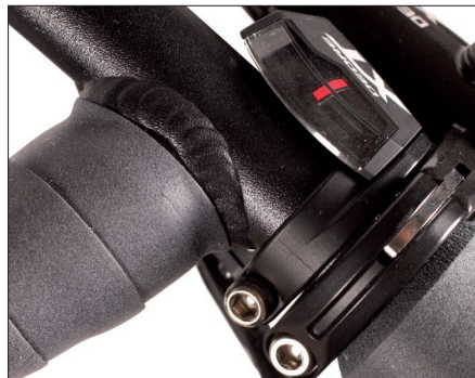
Above, correct lever position on aluminium H-Bar™
